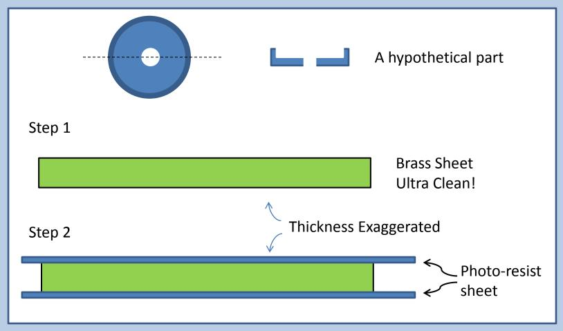
Laminate Photo-resist sheet on both sides
