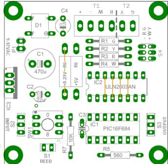
6. Insert the small 0.1 ceramic capacitor (C3 "104") and bend the leads to hold it in place.
