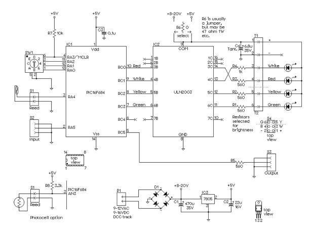
The schematic diagram shows the block signal controller with both the timer and prototypical options. Outputs are configured for a B&O signal. The PIC microcontroller is at the left, the driver transistor array is at the right, and the five volt power supply is at the bottom.
